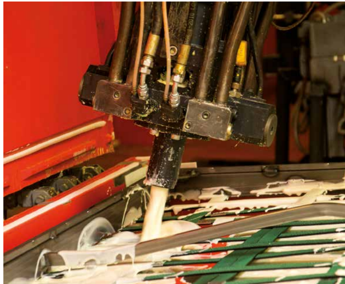
B&B Italia production, Novedrate. Cold polyurethane injection.
